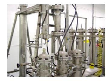
Pilot Plant Supercritical Fluid Extractor
